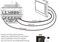
7. If the light is controlled by the live wire and the neutral wire:
