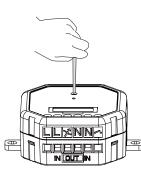
To set the device into pairing mode use the pin to press the button for 2 seconds. The device will then go into pairing mode.
