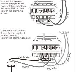
5. Wall installation Remove the existing wall switch. This receiver is a replacement for the existing wall switch and it is not suitable if the existing light switch is interconnected to the other light switches for multi way switching. Do not exceed the maximum load: 300W. 6.Connect the live wire and switch wire: Connect the live wire to the [L] contact. Connect the switch wire to the | contact.
